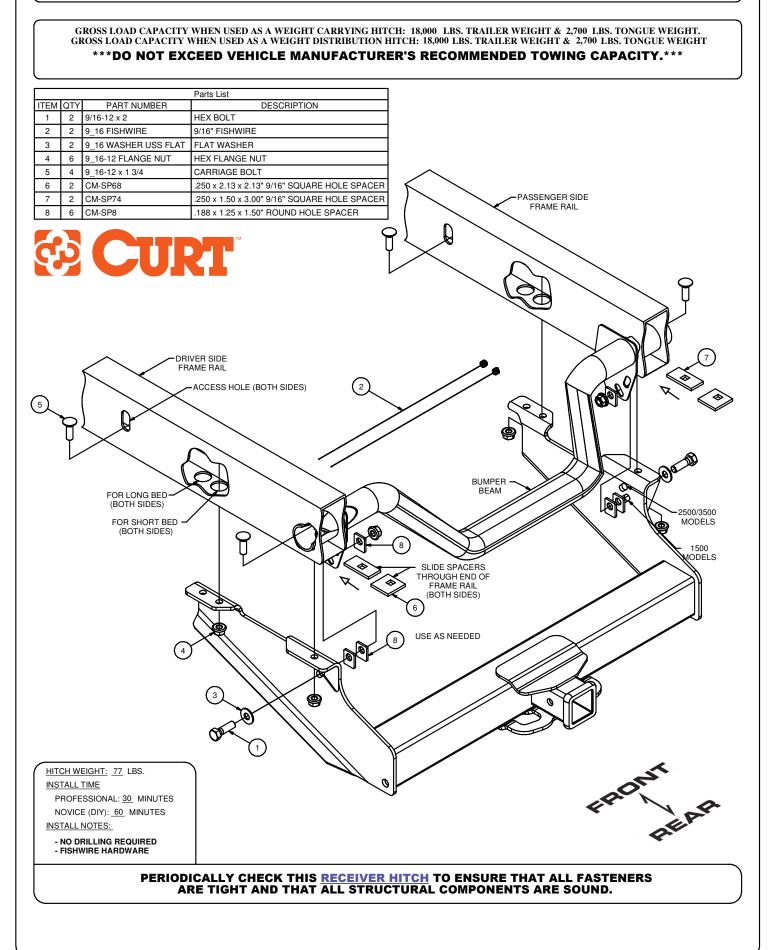
03-CURRENT DODGE RAM 2500/3500 WITHOUT OEM RECEIVER 03-08 DODGE RAM 1500 BUILT AFTER NOV. 2002 WITHOUT OEM RECEIVER
