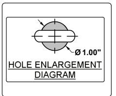
4. Fishwire CM-SP2 spacers and 7/16" carriage bolts through enlarged holes and out forward mounting holes. Reverse fishwire CM-SP2 spacers and 7/16" carriage bolts into enlarged holes.
