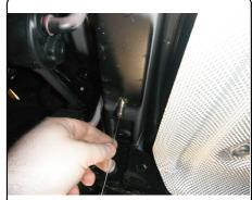
5. Raise hitch into position and secure with 7/16" hex flange nuts.
