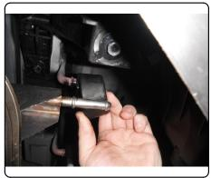
2. Using a 10mm socket, remove plastic fascia tab supports attaching fascia tab to bottom of frame rails on driver and passenger corners of vehicle. Return both supports and (2) support screws to vehicle owner. Retain the remaining (2) support screws for reinstallation.
