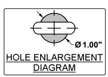
4. Fishwire CM-SP2 spacers and 7/16" carriage bolts through enlarged holes and out forward mounting holes. Reverse fishwire CM-SP2 spacers and 7/16" carriage bolts into enlarged holes.
