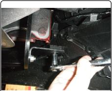
8. Raise exhaust back into position and reattach all exhaust hangers.
