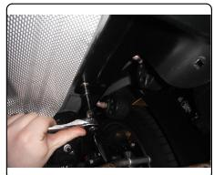
6. Attach 11435-FT brackets to hitch side plates using 1/4" carriage bolts and 1/4" nylock nuts, as shown. Attach driver and passenger side vehicle fascia tabs to 11435-FT brackets using the existing M6 fascia support screws.
