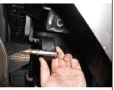
2. Using a 10mm socket, remove plastic fascia tab supports attaching fascia tab to bottom of frame rails on driver and passenger corners of vehicle. Return both supports and (2) support screws to vehicle owner. Retain the remaining (2) support screws for reinstallation.
