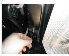
5. Raise hitch into position and secure with 7/16" hex flange nuts.
