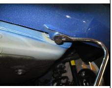
2. Remove one (1) M8 bolt on passenger side frame rail using a 13mm socket. Pull plastic away from frame rail as shown in photo below.
