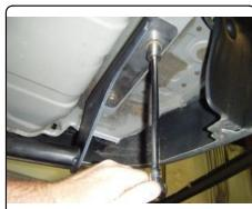
4) Raise exhaust back into location and reinstall rubber isolator.
