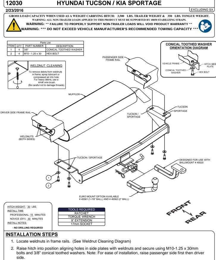
3. Torque all M10 fasteners to 48 ft-lbs.
