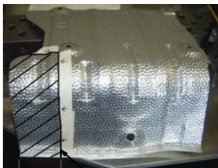
3-1/2" AREA TO TRIM HEAT SHIELD TRIMMING DIAGRAM
