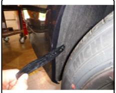
2. Remove (1) screw hidden behind the wheel well at the top of the facia. Remove the plastic clip by prying it out with a flat head screw driver.
