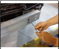
10. Reinstall bumper cover by reassembling components removed in STEPS 1-6 in reverse order.
