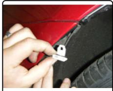
3. Remove small plastic panel between tail light and trunk opening. Remove exposed screw.
