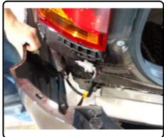
6. Remove foam and set aside for reinstall later.
