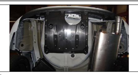
2. Raise hitch into position and align the holes in the side plates with the weldnuts in the frame rails. Secure the hitch using M12-1.25 x 30mm hex bolts and 1/2" conical toothed washers.
