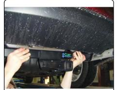
5. Secure hitch to vehicle with (4) 1/2" flange nuts.
