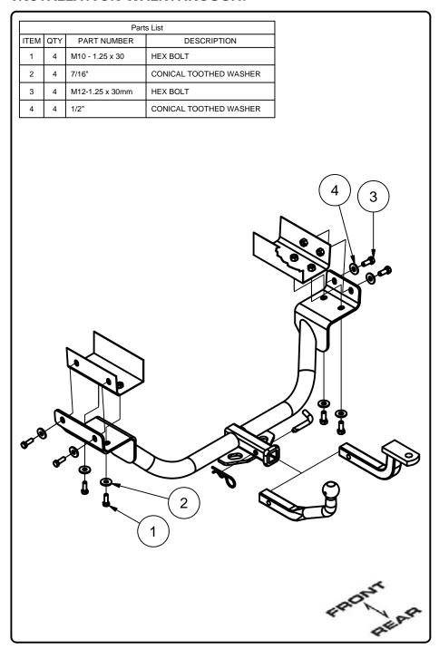
1. Remove existing tow loop from passenger side of vehicle. Return tow loop and hardware to vehicle owner.
