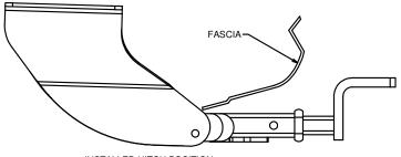
INSTALLED HITCH POSITION
