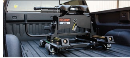
Chevrolet / GMC roller adapter installed in a short-bed truck with A20 head and R20 roller kit (16669)
