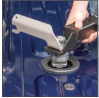
Step 1 - Drop OEM product into the truck bed puck system
