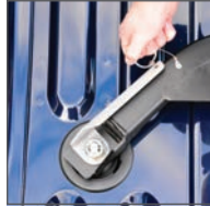
Step 3 - Secure levers with attached safety pins
