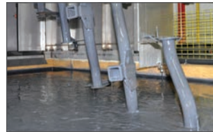
Liquid Bonderite® applied inside and out for max rust resistance
