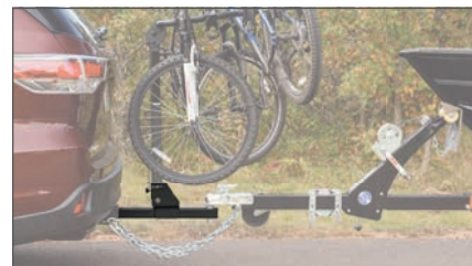
Towable shank allows use of the bike rack while towing a trailer, see page 353 for details
