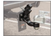
Ball & pintle combo attached to coupler
