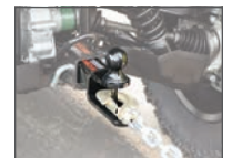
Clevis pin accepts hook or strap for straight-line pull
