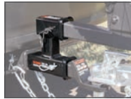
45792 provides two receiver tubes
