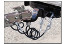
Safety cables in use
