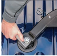
Step 2 - Close the anchor levers to lock roller into place
