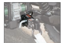
Converts an ATV platform into a 2" receiver tube
