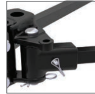
Pin-style spring bars improve strength
