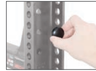
Built-in anti-rattle prevents shaking (45900)
