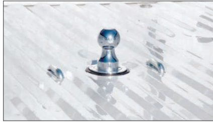
B Using brackets and a gooseneck head
