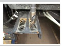
Slide the baseplate (#1, #2) on top of the frame and align with the existing front tow hook holes. Install two of the 5/8" x 1-3/4" hex head cap screws (#6) and washers into the holes previously enlarged. Secure with 5/8" serrated flange nuts (#8).
