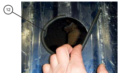
U-EDGING INSTALLED AROUND EDGE OF 4" HOLE IN TRUCK BED
