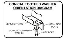
PERIODICALLY CHECK THIS GOOSENECK HITCH TO ENSURE THAT ALL FASTENERS ARE TIGHT AND THAT ALL STRUCTURAL COMPONENTS ARE SOUND.
