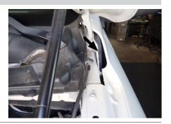
Route the 4-flat along the driver-side inner fender. Mount the 4-flat in the front of the vehicle under the hood.
