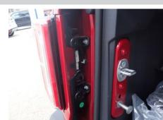
Locate the taillight housing and separate the connectors, taking care not to damage the locking tabs. Repeat this on the other side of the vehicle.
