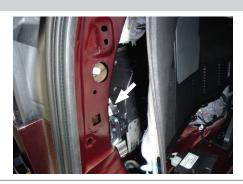
Locate a suitable grounding point near the connector such as an existing screw with nut in the vehicle frame or drill a 3/32" pilot hole for the provided screw. The area should be free of rust, dirt and paint. Secure the white ground wire using the ring terminal and provided screw.
