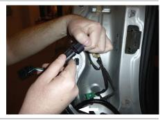
Route the harness so that it drops down just above the driver-side exhaust tip. Locate the harness end with the green wire and route it along the rear bumper. Loosely zip tie in place.
