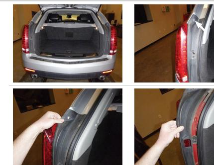
Remove the two Phillips head screws securing the taillight to the vehicle. Carefully remove the taillight by pulling straight back.
