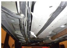
At the front of the fuel tank, find the hard fuel and brake lines. Route the 4-flat along these lines to the rear of the front wheel. Once you have reached the front wheel, route the 4-flat between the vehicle body and the front suspension mount.
