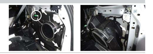
Locate the gray housing similar to that of the custom RV harness. Separate the connectors, taking care not to damage the locking tabs. Insert the custom RV harness end with the green wire between the separated connectors. Make sure the connectors are fully inserted with locking tabs in place.
