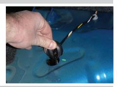
Using a rotary tool, cut a relief in the trunk pan hole just big enough to get the 4-flat through the grommet hole.
