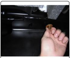
5. Torque all 1/2" fasteners to 110 lb.-ft. and all 12mm fasteners to 86 lb.-ft.
