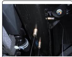
Raise hitch into position and looesly install the (4) 1/2" hex flange nuts supplied. Loosely install the remaining (2) 12mm hex bolts and conical tooth washers supplied.
