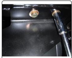
6. Reinstall the skid shield with the fasteners removed in step 1.
