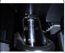
2. Fishwire (2) 1/2" carriage bolts and spacers into the lower mounting locations on the driver side frame rail.
