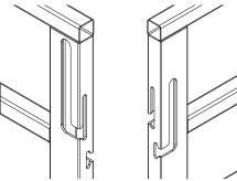
Small slot to be used for vehicles with a 1/2" tailgate pin
