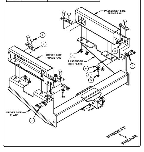
Note: To ease installation, temporary removal of the spare tire is recommended. A 21mm socket will be needed.
