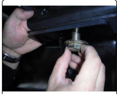
4. Place the 1/2" hex bolts and concial tooth washers into position as shown. Install 1/2" hex flange nuts.
