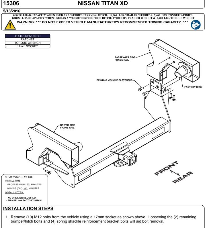
NOTE: Be sure not to strip the threads of any of the bolts removed or loosened.
