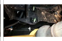
4. Locate and remove the (3) factory M14 bolts on the outside of the driver side frame rail and (1) M14 from the underside of the frame. Repeat on the passenger side frame rail to remove the factory hitch. Save hardware for reinstallation.
