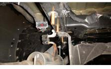
7. Raise hitch into position. Secure hitch to the vehicle frame using 1/2" hex flange nuts. Reinstall short factory M14 bolt removed earlier to finish securing the hitch to the frame on each side of the frame.
