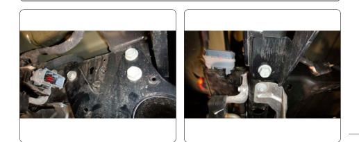
5. Remove (2) factory M6 bolts from the passenger side and (1) M6 bolt on the driver side from the exhaust heat shield. Using a hammer, flatten the heat shield tabs against the frame, heat shield tabs will be pinched between the hitch side plates and the frame.
