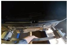
Gently bend the two fascia mounting tabs rearward to allow clearance for the trailer hitch.
