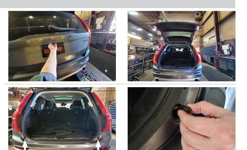
Gently pull enough of the wheel well trim out to remove the rear fascia on both sides of the vehicle. Gently remove the rear bumper fascia by pressing the three clips on the rear bumper fascia on each side, gently pulling the rear bumper fascia off the vehicle, and unplugging one or two connectors from fascia.
