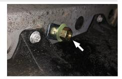
Using a 14mm socket, tighten the bumper nuts on each side of the vehicle to 33.4 lb-ft.
