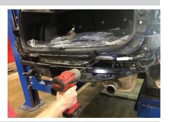
Lower the muffler by removing the two rearmost rubber exhaust hangers.
