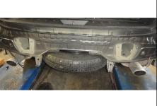
9. Using a hammer, bend bumper mounting flange inward toward the front of the vehicle to allow hitch to mount flush with vehicle.
