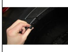
5. Open the liftgate. Remove panel near taillight on both sides of the vehicle by pulling straight back from the top of the panel, allowing access to the (1) bolt that connects the fascia to the vehicle body. Remove this bolt from each side using a 10mm socket to allow fascia to be removed. Set panel and hardware aside for reintallation in STEP 11.
