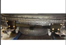
11. Reinstall fascia removed in STEPS 1-6 in reverse order. Be sure to reconnect the plugs that were disconnected during fascia removal process. <u>Note:</u> fascia has a removable panel for hitch usage. The panel can then be reinstalled when hitch is not in use.
