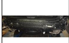
7. Remove (2) wire harnesses from bumper. The harnesses are located on the top of the bumper beam. <u>Note:</u> Using the pry tool may be helpful.
