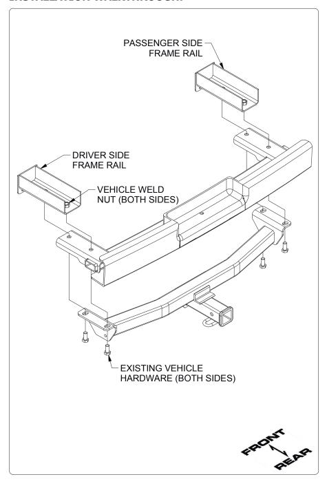
1. Clamp bumper assembly in position. Remove (4) M16 bolts, (2) on each side.
