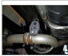
4. Locate and remove (2) plastic nuts with a 10mm socket. Remove heat shield and mark out a 5" x 13" section with masking tape. Use aviation shears to trim marked area. Reinstall with (1) nut using a 10mm socket. NOTE: If no underbody panel, remove (4) plastic nuts, trim panel, and reinstall with (3) plastic nuts.
