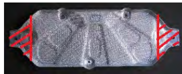
HEAT SHIELD TRIM DIAGRAM
