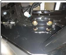
2. Torque 12mm fasteners to 86 lb-ft.
