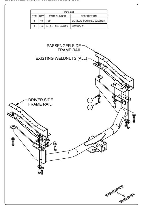
1. If present on vehicle remove tow hooks before installing hitch and return hooks and hardware to vehicle owner. Raise hitch into position. Fasten hitch by threading (10) M12 x 40mm bolts with conical washers into existing weld nuts as shown.
