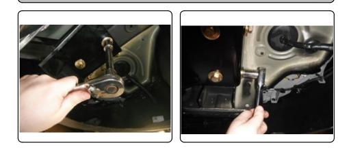
5. Raise exhaust back into position and reattach exhaust isolators removed in Step 2.
