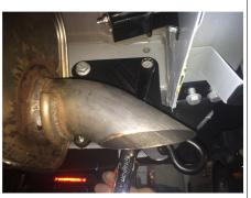
2. Raise hitch into position and loosely fasten provided hardware. Use 3/4" socket to torque all 1/2" fasteners to 110 ft-lbs.
