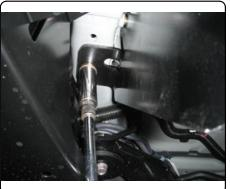
6. Reinstall canister fastener, if removed, and rubber exhaust hangers.
