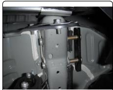
4. Raise hitch into position and slide the bolts through to support it. Loosely install the supplied hex flange nuts and the (2) hex bolts and conical washers as shown. Be sure teeth on washers are against the hitch mounting plate.
