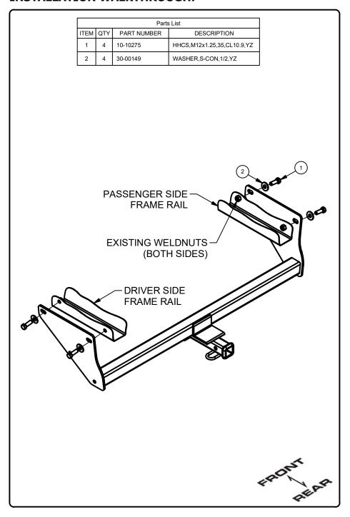
1. Remove stickers covering holes on the outside of the frame rails. If equipped, remove tie down bracket from bottom of passenger side frame rail and return to vehicle owner.
