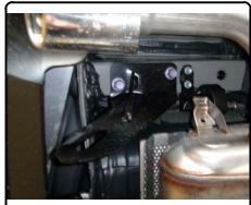
2. Raise hitch into position and secure with supplied M12 bolts and 1/2" conical tooth washers. Torque M12 hardware to 86 ft-lbs.
