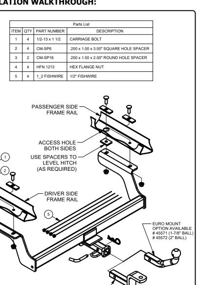
DESIGNED FOR USE WITH BALL MOUNT # 45521 1. Remove (2) rubber plugs from each frame rail and return to vehicle owner (leave center plugs in the frame).
