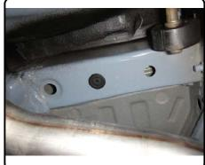
2. Enlarge access holes and fishwire 1/2" carriage bolts and CM-SP6 spacers into position and reverse fishwire remaining 1/2" carriage bolts and CM-SP6 spacers into access hole. Leave fishwires attached.
