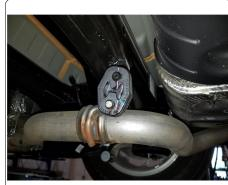
4. Locate and remove (2) plastic nuts with a 10mm socket. Remove heat shield and mark out a 5" x 13" section with masking tape. Use aviation shears to trim marked area. Reinstall with (1) nut using a 10mm socket. <u>NOTE</u>: If no underbody panel, remove (4) plastic nuts, trim panel, and reinstall with (3) plastic nuts.
