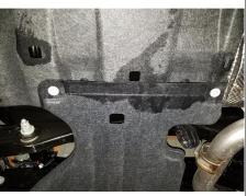
2. Locate and remove (3) screws from driver side wheel well with an 8mm socket. Remove underbody panel and mark out a 0.5" x 10" slot with masking tape. Use aviation shears to trim underbody panel. Set aside for later reinstallation.
