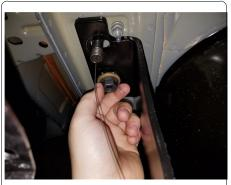
10. Torque all 1/2" hardware to 110 ft-lbs. Reinstall Underbody panel following steps 1 and 2 in reverse order.
