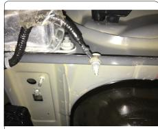
9. Raise hitch into position starting with the passenger side. Run the fishwires through the holes on hitch to help align bolts with hitch holes. Remove fishwires and loosely fasten (2) 1/2" hex flange nuts on driver side and (3) 1/2" hex flange nuts on passenger side.
