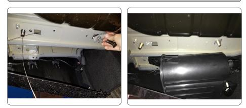
8. On driver side frame rail locate and remove (1) nut using 10mm socket.
