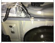
9. Raise hitch into position starting with the passenger side. Run the fishwires through the holes on hitch to help align bolts with hitch holes. Remove fishwires and loosely fasten (2) 1/2" hex flange nuts on driver side and (3) 1/2" hex flange nuts on passenger side.
