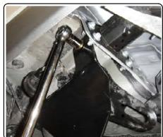
4. Raise exhaust and reinstall the rubber isolators.
