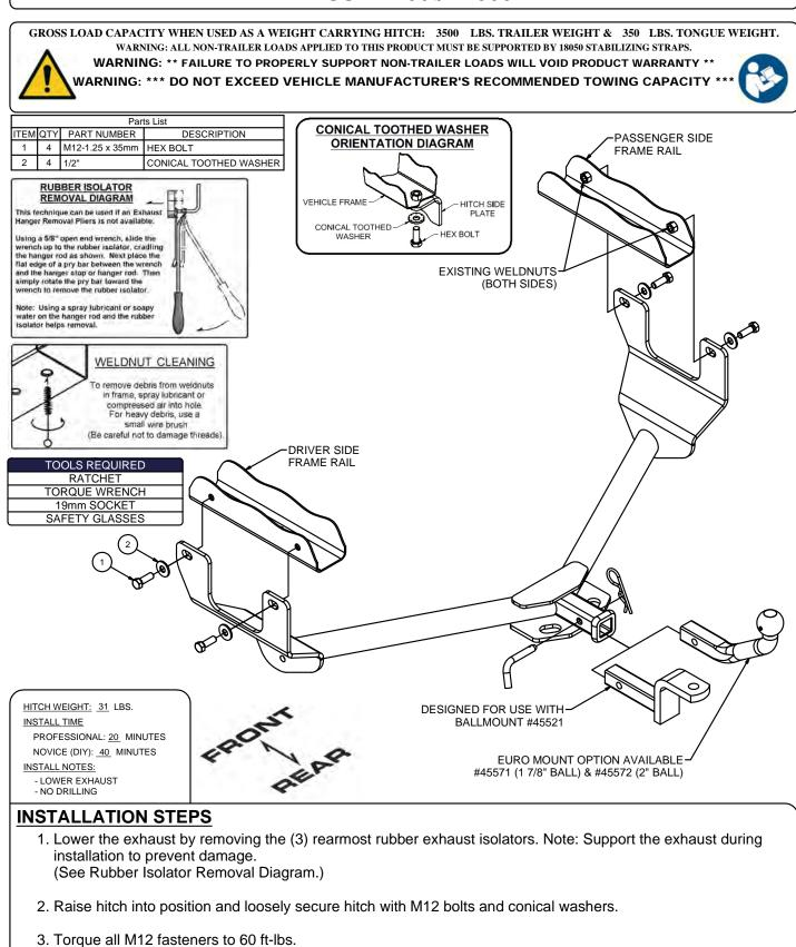
4. Raise exhaust and reinstall the rubber isolators.
