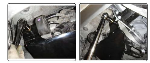
4. Raise exhaust and reinstall the rubber isolators.
