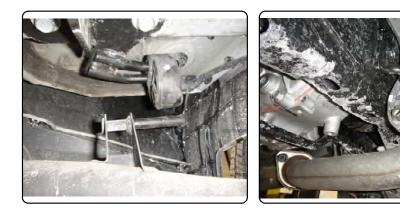
2. <u>Raise hitch into position</u> and loosely secure hitch with M12 bolts and conical washers.
