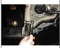
5. Raise exhaust back into position and reattach exhaust isolators removed in Step 2.
