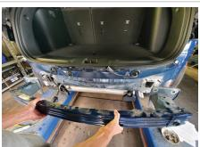
Raise the trailer hitch into position over the existing M10 screws on both sides of the vehicle. Place the bumper beam over hitch.
