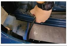
If applicable, remove all electrical connectors from the frame. Trim the caulk around the bumper beam on both sides. You will be reinstalling the electrical connectors in Step 10.
