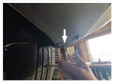
On the driver side, open the two access covers to reveal the taillight screws. Unscrew the two screws and gently pry on the fascia. Remove the taillight by pulling rearward on both sides of the light. Set the screws and taillight aside for reinstallation in Step 10.
