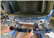
Raise the trailer hitch into position over the existing M10 screws on both sides of the vehicle. Place the bumper beam over hitch.
