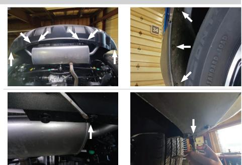
On the driver side, open the two access covers to reveal the taillight screws. Unscrew the two screws and gently pry on the fascia. Remove the taillight by pulling rearward on both sides of the light. Set the screws and taillight aside for reinstallation in Step 10.
