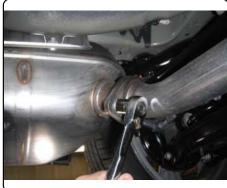
2. Remove the rearward most screw in the heat shields on the frame rail. Measure 5" forward on the heat shield and make a 1.25" hole in line with the screw hole (both heat shields). Flattening the heat shield around the screw that was removed will aid in installing the forward most flange nuts.
