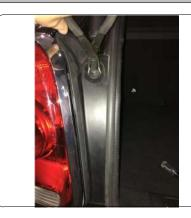
5. Remove (2) bolts from each tail light using 10mm socket. Carefully remove tail light from vehicle and unclip electrical harness.
