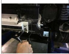
8. Raise hitch into position using studs to align. Reinstall rear bumper beam over hitch and secure using existing vehicle hardware.
