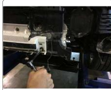
8. Raise hitch into position using studs to align. Reinstall rear bumper beam over hitch and secure using existing vehicle hardware.
