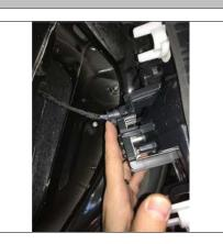
6. Remove rear fascia by locating and removing fastener behind wheel well trim using T25 socket and unclip rear fascia attachments.
