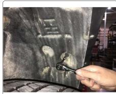
Open rear hatch to expose and remove plastic cover located inbore of each tail light, remove (1) fastener on each side using needle nose pliers.
