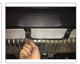
2. Remove (6) rivets along wheel well trim above each rear tire using a small punch and pry tool.
