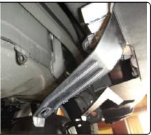
2. <u>Raise hitch into position</u> and install supplied fasteners as shown. Torque all 3/8" fasteners to 45 lb-ft and all 5/8" fasteners to 210 lb feet. Re-install remaining bumper fascia tabs to original positions.
